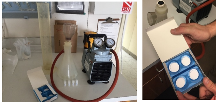
Figure 2. Complete vacuum set up with funnel, Erlenmeyer flask, graduate cylinder and filters (left) and box of Whatman GF/F filters (right).
